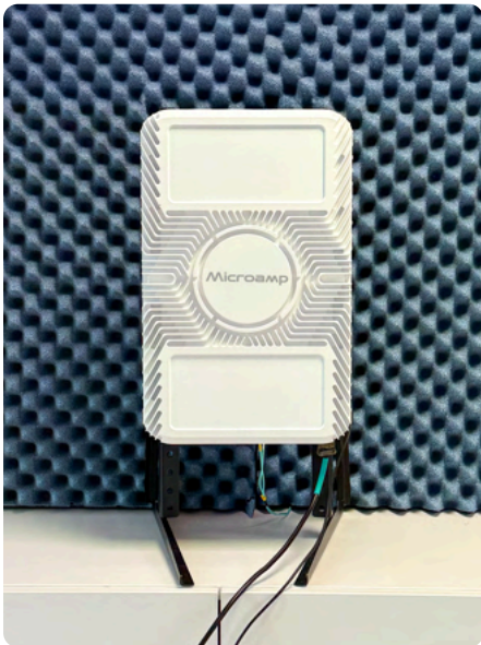
Photo 1: Microamp 5G mmWave CellBox Air radio
